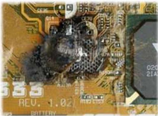
Figure 2 capacitor burned by 2kHz-150kHz emissions
